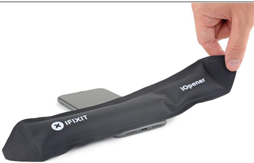
ⓘ Heating the lower edge of the iPhone helps soften the adhesive securing the display, making it easier to open.
